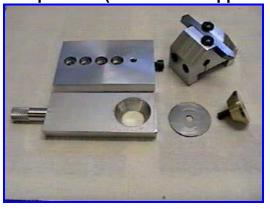
**Base:** Aluminum, ½" x 2-1/2" x 4". SHCS in the end locks the Pivot mounting/adjustment screw.
