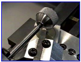
( Note the size and angle of the relief notch on the tool holder. I cogitated on this way too long and finally accepted the idea that the diameter and angle would be "right on" for one, and only one, setup. This ain't it. But, it worked out just fine in all the variations I tried.
